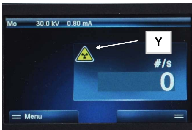
Fig. 10: Screen for controlling the unit at the front of the unit. The x-radiation is not activated.
