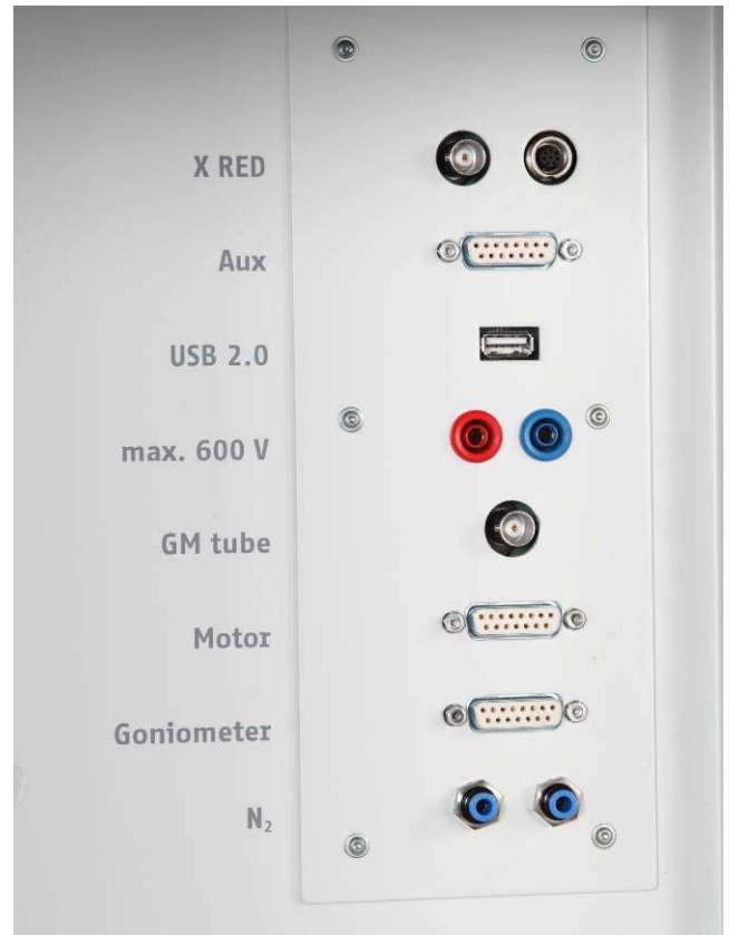
Fig. 7: Socket panel inside the experiment chamber
